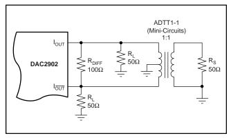
FIGURE 3. Differential Output Configuration Using an RF Transformer.
