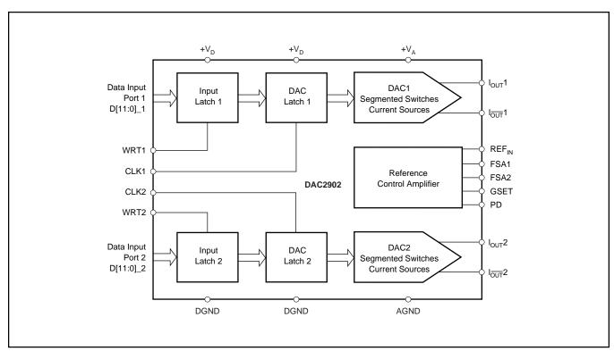
FIGURE 1. Block Diagram of the DAC2902.
