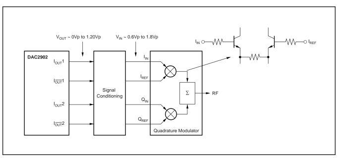
FIGURE 7. Generic Interface to a Quadrature Modulator. Signal Conditioning (Level-Shifting) May Be Required to Ensure Correct DC Common-Mode Levels At the Input of the Quadrature Modulator.
