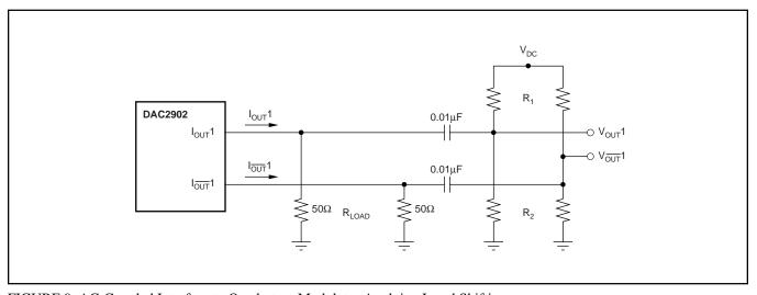
FIGURE 9. AC-Coupled Interface to Quadrature Modulator Applying Level Shifting.
