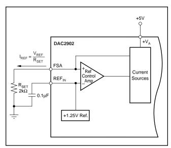
FIGURE 10. Internal Reference Configuration.
