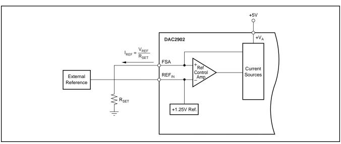
FIGURE 11. External Reference Configuration.
