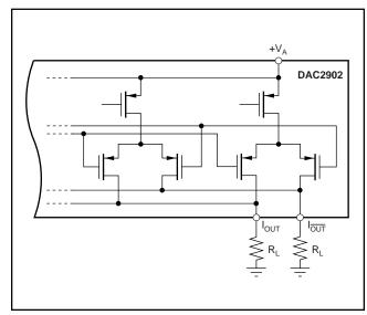
FIGURE 2. Equivalent Analog Output.
