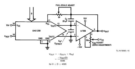
FIGURE 9. Unipolar Output Configuration
