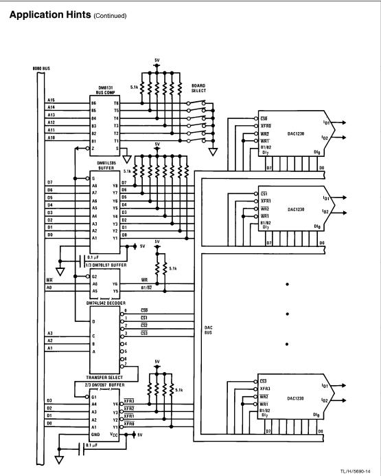
FIGURE 8. TRI-STATE® Buffers Isolate the Data and Control Lines from the DACs.
