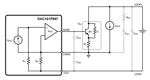
Figure 16. Capacitances affecting Control Loop
