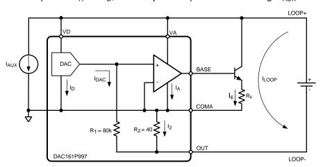
Figure 13. Loop-Powered Transmitter
