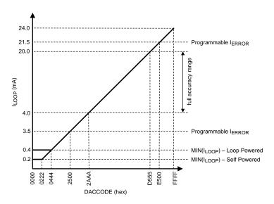
Figure 15. DAC DC Transfer Function
