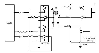
Figure 27. Master without Bidirectional I/O
