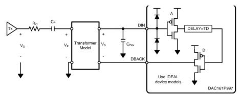
Figure 32. NRZ Waveform Transmission and Recovery Circuit Model
