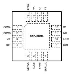
Figure 1. WQFN-16 (RGH0016A) Top View
