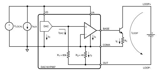
Figure 14. Self-Powered Transmitter
