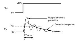
Figure 33. SWIF Link Circuit Response to Step Input
