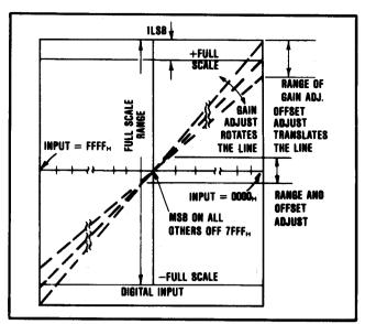
FIGURE 2. Relationship of Zero and Gain Adjustment.
