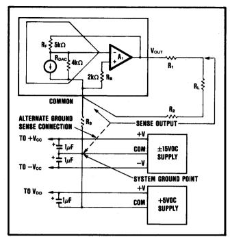
FIGURE 3. Output Circuit.
