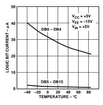
Figure 15. Digital Input Current vs. Temperature
