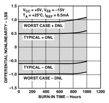
Figure 16. Differential Nonlinearity vs. Time Accelerated by Burn-In
