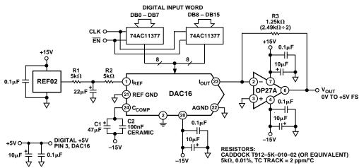
Figure 26. DAC16 Noise Measurement Test Circuit
