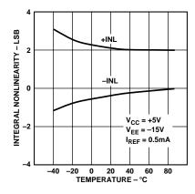
Figure 11. Integral Nonlinearity vs. Temperature
