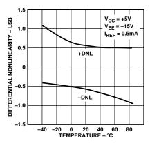
Figure 12. Differential Nonlinearity vs. Temperature
