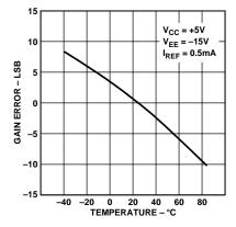
Figure 10. Gain Error vs. Temperature
