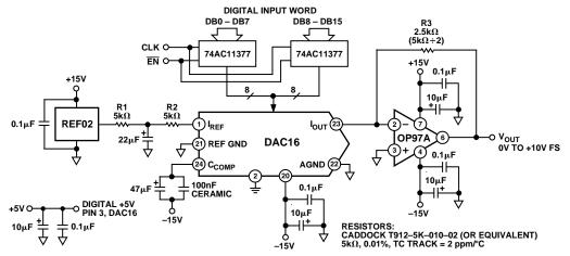
Figure 24. Unipolar Circuit Configuration
