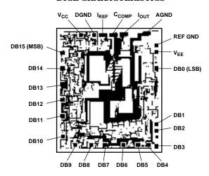
Die Size  $0.129 \times 0.153$  inch, 19,737 sq. mils  $(3.277 \times 3.886 \text{ mm}, 12.73 \text{ sq. mm})$ The DAC16 Contains 330 Transistors. Substrate is  $V_{EE}$  Polarity.
