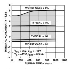
Figure 17. Integral Nonlinearity vs Time Accelerated by Burn-In
