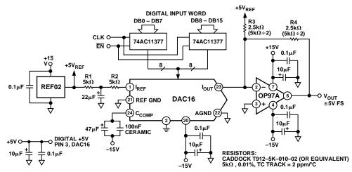
Figure 25. Bipolar Circuit Configuration
