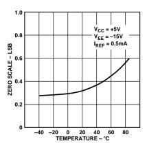
Figure 9. Zero Scale Output vs. Temperature
