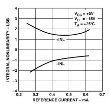
Figure 7. Integral Nonlinearity vs. I<sub>REF</sub>
