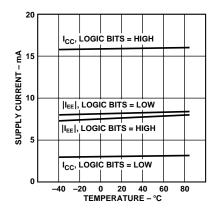
Figure 13. Supply Current vs. Temperature
