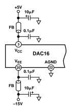
Figure 20. Using a Ferrite Bead as a High Frequency Filter
