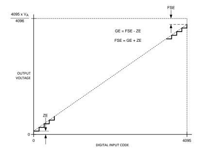
Figure 3. Input / Output Transfer Characteristic
