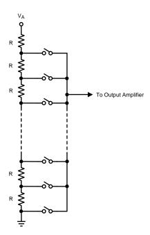
Figure 33. DAC Resistor String
