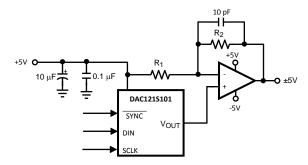
Figure 43. Bipolar Operation
