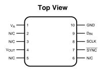
Figure 1. 10 Lead CLGA Package See Package Number NAC0010A
