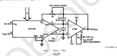
FIGURE 9. Unipolar Output Configuration
