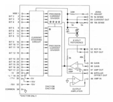
Figure 1. Block Diagram and Pin Designations
