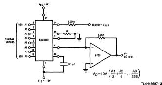
FIGURE 1. + 10V Output Digital to Analog Converter (Note 7)
