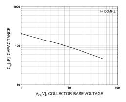
Figure 3. Collector Output Capacitance
