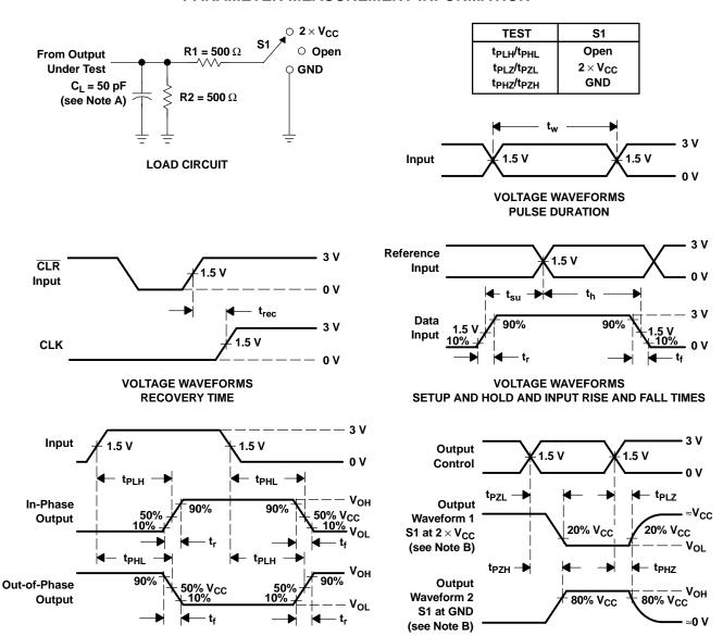
NOTES: A.  $C_L$  includes probe and test-fixture capacitance.
