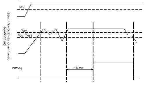
Figure 8. Timing for Customer Test Mode
