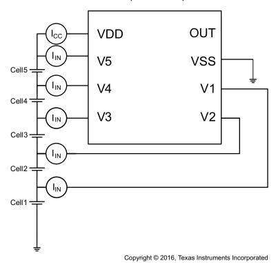
Figure 10. Configuration for IC Current Consumption Test
