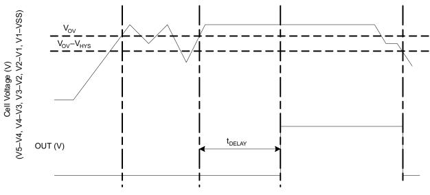
Figure 7. Timing for Overvoltage Sensing
