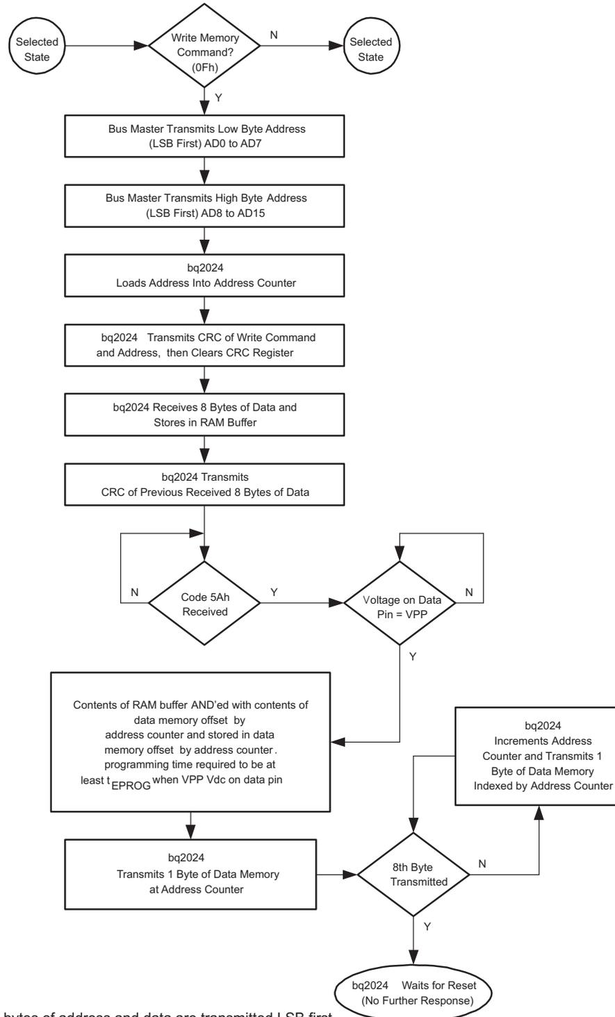
NOTE: Individual bytes of address and data are transmitted LSB first
