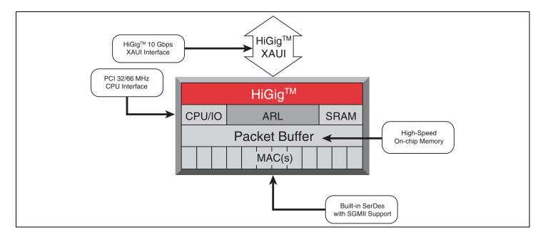
The BCM5692 network switch is a scalable, modular chip solution with 12 ports. Each of these flexible ports supports Gigabit Ethernet or 10/100-Mbps Ethernet. Additionally, the BCM5692 supports both copper and fiber physical interfaces. The BCM5692 has a fully integrated SerDes functionality consisting of a 10-Gbps XAUI HiGig Port, Gigabit Ethernet, or SGMII PHY interface.
