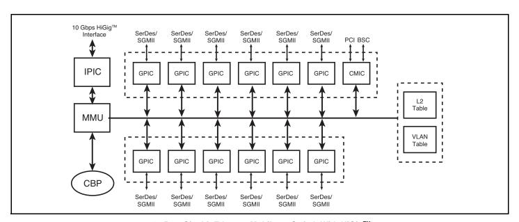
12-Port Gigabit Ethernet Multilayer Switch With HiGig™
