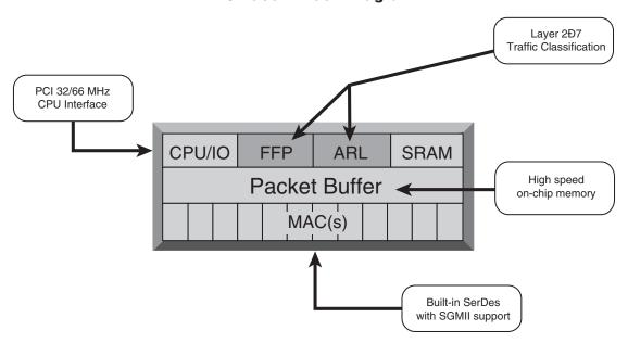
The **BCM5691** network switch is a scalable, modular chip solution with 12 ports. Each of these flexible ports supports Gigabit Ethernet or 10/100 Mbps Ethernet. Additionally, the **BCM5691** supports both copper and fiber physical interfaces. The **BCM5691** has a fully integrated SerDes functionality consisting of a Gigabit Ethernet or a SGMII PHY interface.
