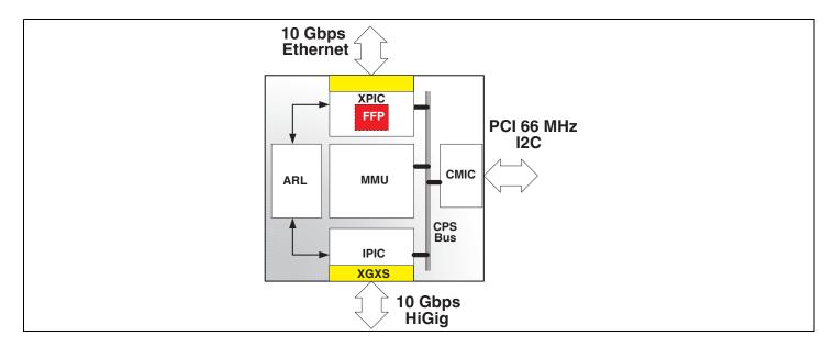
The BCM5673 10 Gigabit Ethernet switch is a scalable, multi-layer switch-on-chip member of the StrataXGS family. The BCM5673 is a dual port switch, which supports a 10 Gigabit Ethernet (IEEE802.3ae) port and a HiGig™ uplink port. The 10 Gigabit Ethernet port can be used to interface to the XENPAK module via the XAUI interface.
