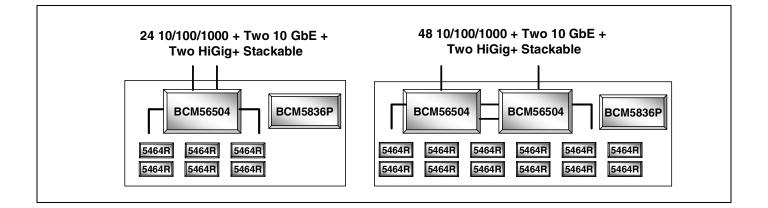
The BCM56504 is the fifth generation of the highly-integrated and costeffective StrataSwitch and StrataXGS product line. The BCM56504 is a single-chip solution with 24-GbE ports and four 10-GbE/HiGig+ uplink ports.
