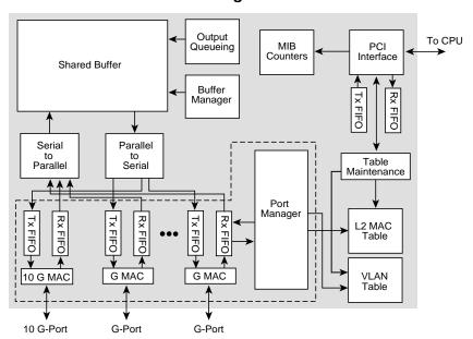
The **BCM5632** switching processor chip supports 12 Gigabit ports and one 10-Gigabit uplink with all ports in wirespeed operation. The BCM5632 is ideal for applications such as multi-Gigabit port switches or aggregating multiple-Gigabit ports to a 10-Gigabit backplane.
