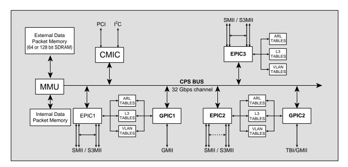
The **BCM5616**, with a forwarding rate of 6.6 Mpps, defines the next generation of performance for single-chip switching solutions. Through its advanced ContentAware<sup>TM</sup> feature set, the StrataSwitch II product family supports advanced applications and services, at wire speed, with non-blocking performance.
