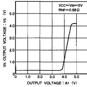
Fig.10 Vs output voltage vs. A1 output voltage
