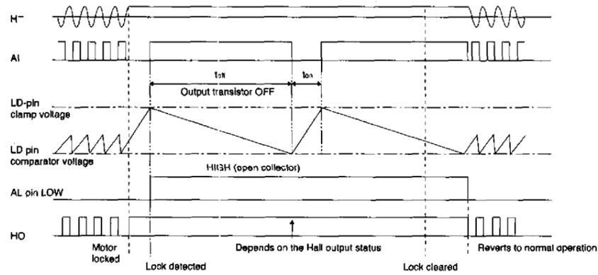
Fig.1 Timing chart for motor locking
