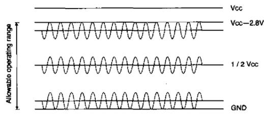
Fig.4 Hall amplifier input bias voltage
