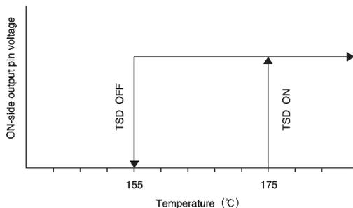
Fig.3 Temperature setting of the thermal shutdown circuit
