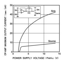
Fig.7 Op-amp maximum output current characteristics
