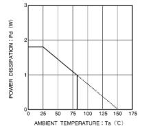
Fig.3 Thermal derating curve
