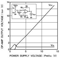
Fig.8 Op-amp saturation voltage characteristics
