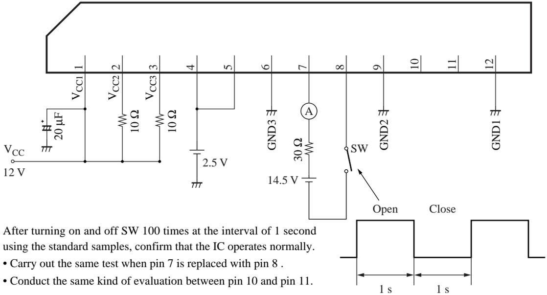
After turning on and off SW 100 times at the interval of 1 second using the standard samples, confirm that the IC operates normally.
