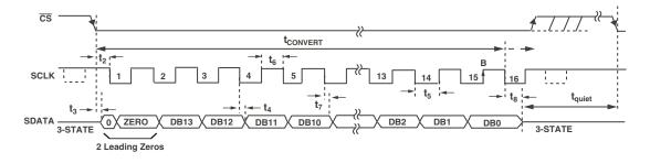
Figure 10. AD7940 Serial Interface Timing Diagram
