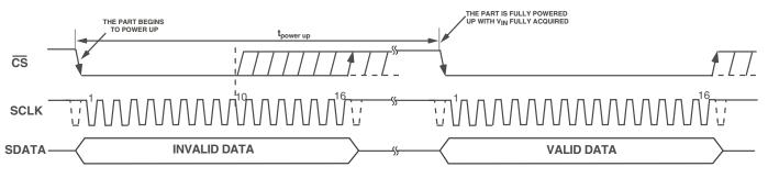
Figure 9. Exiting Power Down Mode
