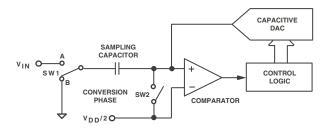
Figure 3. ADC Conversion Phase
