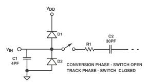
Figure 4. Equivalent Analog Input Circuit
