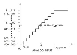
Figure 5. AD7940 Transfer Characteristic
