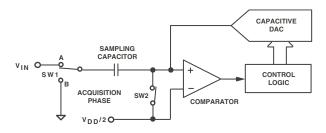
Figure 2. ADC Acquisition Phase
