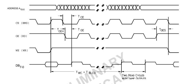
Figure 28. Toggle Bit Timing
