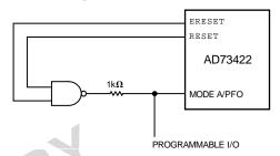
Figure 20. Mode A Pin/EZ-ICE Circuit
