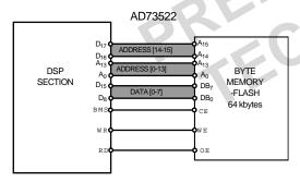
Figure 22. Flash Interface to DSP section
