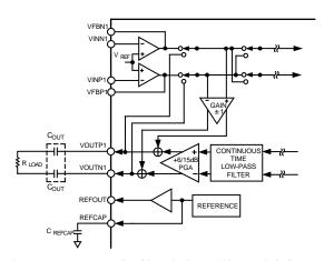
Figure 31. Example Circuit for Differential Output
