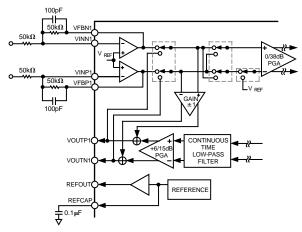
Figure 26. Analog Input (DC-Coupled) Using Internal Amplifiers
