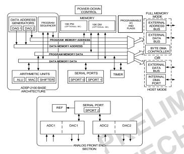
Figure 12. Functional Block Diagram
