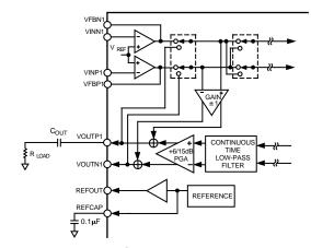
Figure 32. Example Circuit for Single-Ended Output
