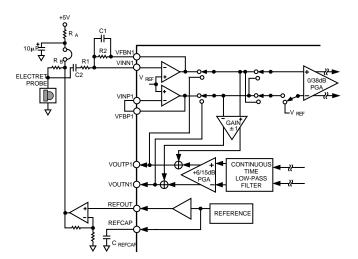
Figure 30. Electret Microphone Interface Circuit
