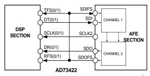
Figure 11. Directly Coupled or Frame Sync Loop-Back Configuration
