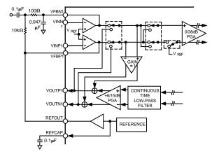
Figure 28. Analog Input (AC-Coupled) Single-Ended
