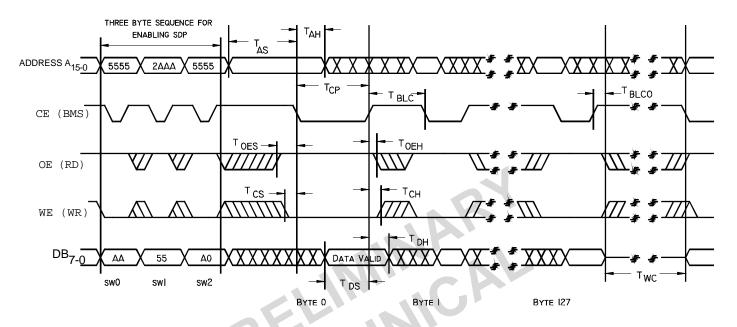
Figure 26. BMS Controlled Page Mode Write Cycle Timing
