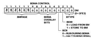
Figure 18. BDMA Control Register
