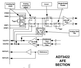
Figure 7. Analog Input/Output Section
