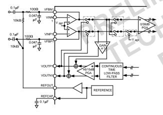
Figure 27. Analog Input (AC-Coupled) Differential
