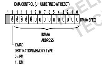
Figure 19. IDMA Control/OVLAY Registers
