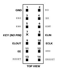
Figure 21. Target Board Connector for EZ-ICE
