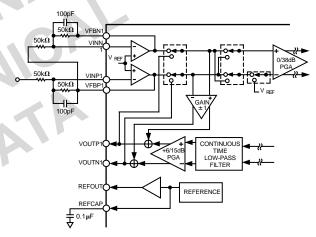
Figure 29. Single-Ended to Differential Conversion On Analog Input
