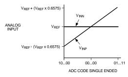
Figure 6. ADC Transfer Function
