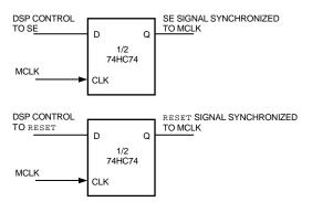
Figure 22. SE and RESET Sync Circuit for Cascaded Operation
