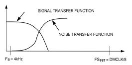
b. Analog Sigma-Delta Modulator Transfer Function
