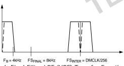
d. Final Filter LPF (HPF) Transfer Function Figure 5. AD73522 ADC Frequency Responses
