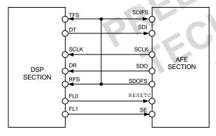
Figure 21. AD73522 AFE to DSP Connection
