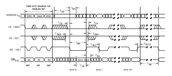
Figure 25. WR Controlled Page Mode Write Cycle Timing
