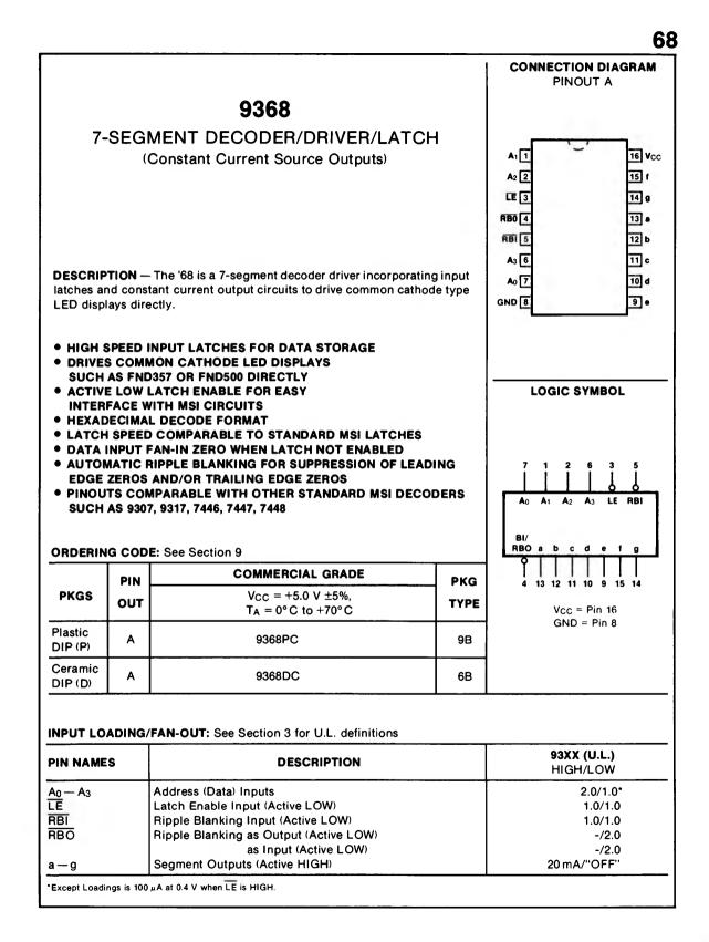
**FUNCTIONAL DESCRIPTION** — The '68 is a 7-segment decoder driver designed to drive 7-segment common cathode LED displays such as the Fairchild FND357 or FND500 directly. The '68 drives any common cathode LED display rated at a nominal 20 mA at 1.7 V per segment without need for current limiting resistors.
