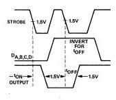
Strobe, P.A. = 2.6V P.W. = 300 ns, 50% to 50% PRR = 1MHz  $t_r = t_f = 5$ ns
