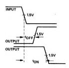
INPUT PULSE: Amplitude = 2.6V P.W. = 30ns, 50% to 50%  $t_r = t_f = 5ns$ PRR = 1MHz
