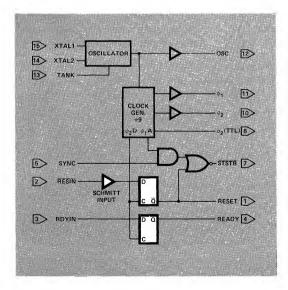
The READY input to the 8080A CPU has certain timing specifications such as "set-up and hold" thus, an external synchronizing flip-flop is required. The 8224 has this feature built-in. The RDYIN input presents the asynchronous "wait request" to the "D" type flip-flop. By clocking the flip-flop with  $\phi$ 2D, a synchronized READY signal at the correct input level, can be connected directly to the 8080A.
