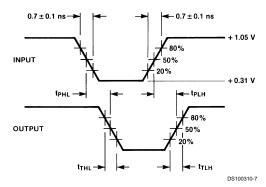
FIGURE 2. Propagation Delay and Transition Times
