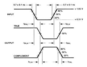
Figure 4. Propagation Delay and Transition Times
