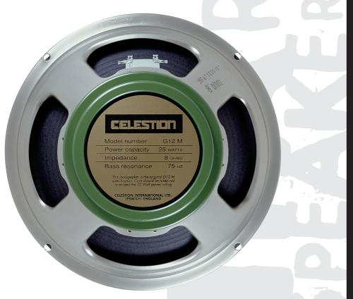
Celestion's first guitar loudspeaker featuring a ceramic magnet structure, the G12M 'Greenback' presented almost as much magnetic flux to the voice coil as an Alnico formulation, but in a much more compact space. As a result the Greenback became the guitar loudspeaker that paved the way for use with higher power amplifiers. And, of course, the ceramic magnet presented its own unique tonal characteristics.
