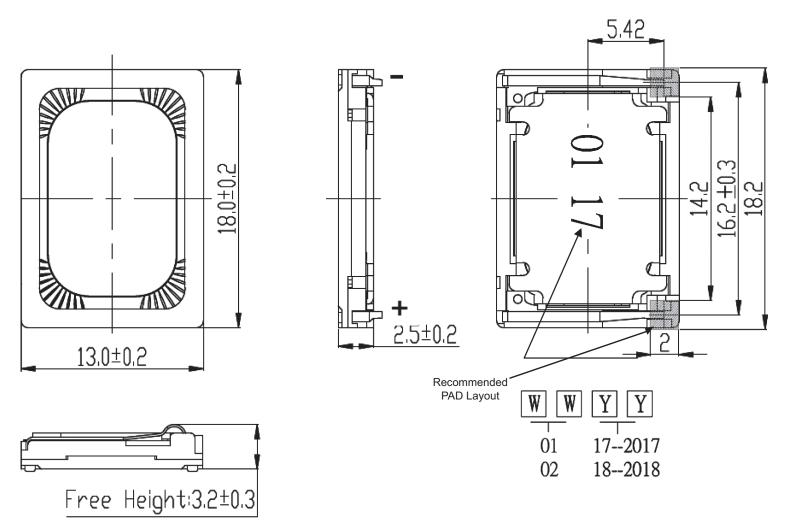
Note: 1. Maximum compression force between front frame and back frame & yoke is 5 N.
