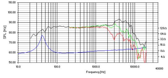
— Impedance— On axis— 30 degree<del>s</del>— 60 degree
