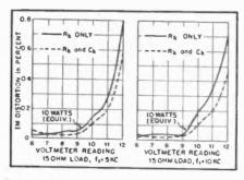
Fig. 9. Effect of capacitor on CCIF intermodulation measurements at two different areas of the frequency spectrum.
