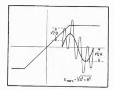
Fig. 8. Graphic representation of possible maximum voltage resulting from mixing two signals of slightly different frequency and of the same amplitude, as in the CCIF method.
