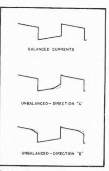
Fig. 11. Effect of current unbalance on square waves. Note that only the low frequency is affected, as indicated by rounding of trailing edge of wave.
