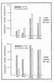
Fig. 5. Comparative distortions with different types of tubes in the output stage show different results.
